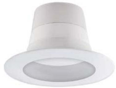
The high brightness Recessed LED uses only 9W and can be the direct retrofit to recessed cans. The Recessed LED fits into an architectural downlight 4" housing providing high performance, energy saving, and long lasting light output. Frosted lens reduces glare to a minimum. Fully dimmable with your regular incandescent dimmer.
